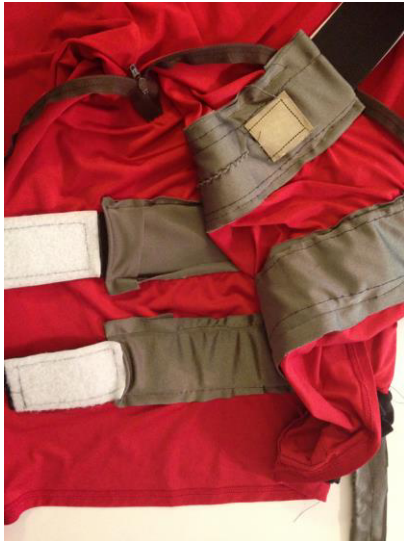
Figure 1: Electrode Integration into Shirt (inside)
